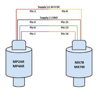
The MX7B/MX7M will now only turn on the cold cathode if the MP2AR/MP4AR detects pressure lower than  $1*10^{-2}$ .
